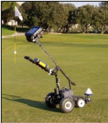
Update system for landscape survey on a motorized cart with individual stand-by power supply
